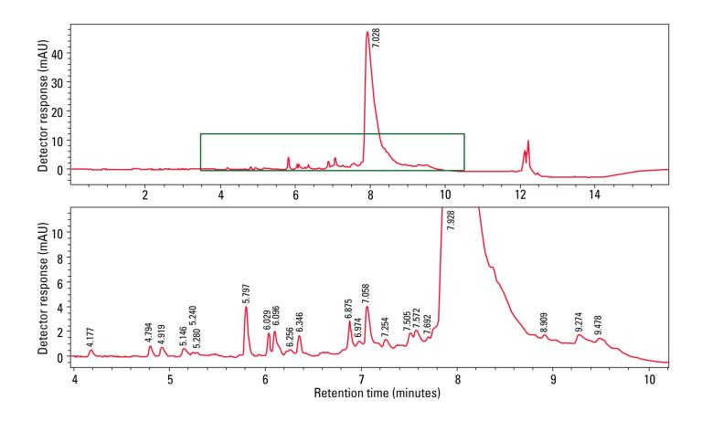
A shallow gradient of 0-15% B in 10 minutes run provides the separation and resolution of oligonucleotide impurities species within a short run time.
